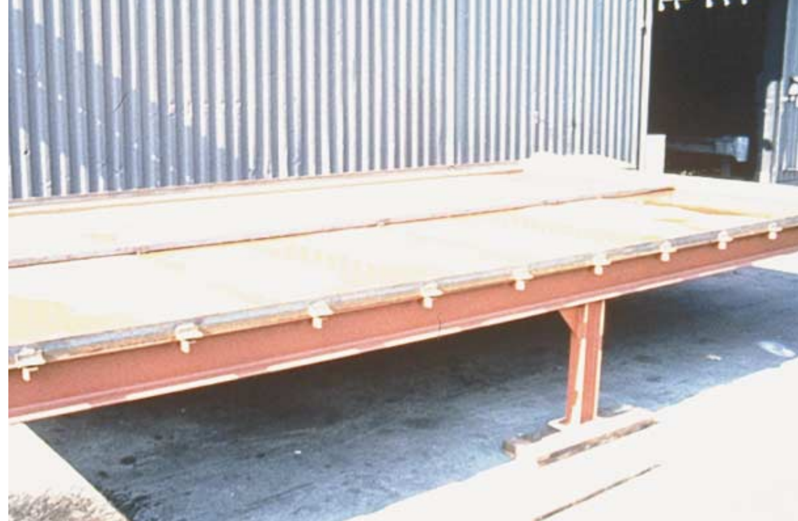
Factory Mutual windstorm classification ratings are determined using a test frame that measures 12-ft. x 24-ft., like the one shown above.
